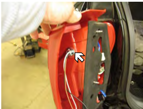
Possible Location of the BX8869 Bulb & Socket Wiring Kit
